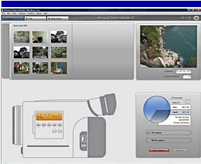
Figure 1: Capture from a DV Camcorder. When connected with a FireWire cable the on-screen mini controls control the Camcorder.
