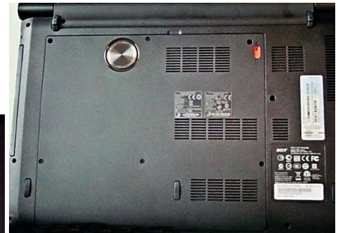
Base showing silver CineBass subwoofer, red slider switch for turning the non-removable battery on and off and screws for access to the HD.
