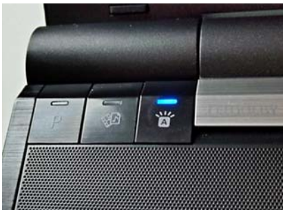
Special shortcut keys. Programmable key (left), Media Centre (centre) and Keyboard backlight (right).
