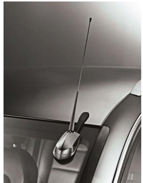
DAB Antenna — Outside View
