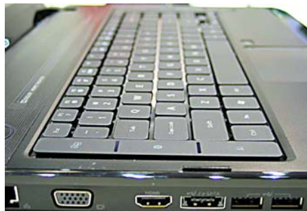
New Acer Aspire 5935 side view showing a versatile selection of connectors: Ethernet, VGA, HDMI, e-SATA & Two USB 2 sockets.
