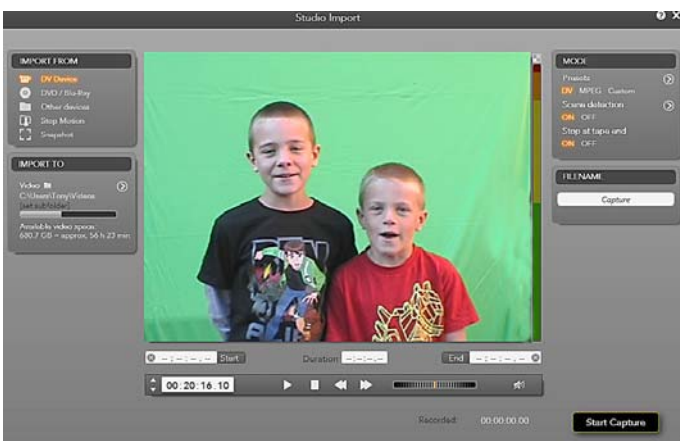
Figure 3: Here I'm importing footage from my DV Camcorder. Controls at the bottom of the picture control the camcorder via the FireWire port on the camcorder. Green screen background shows I'm using it for a chroma-key shot.
