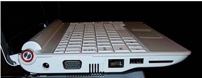
Left Side. Power, External VGA socket, Ethernet, USB2 and SD Card slot
