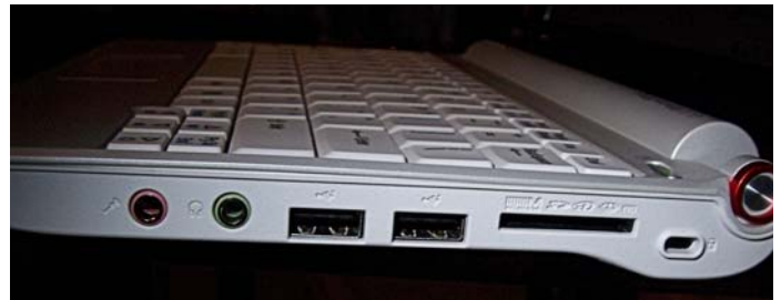
Right Side. Mic. Headphones, 2 x USB2, Memory Card and Kensington Lock
