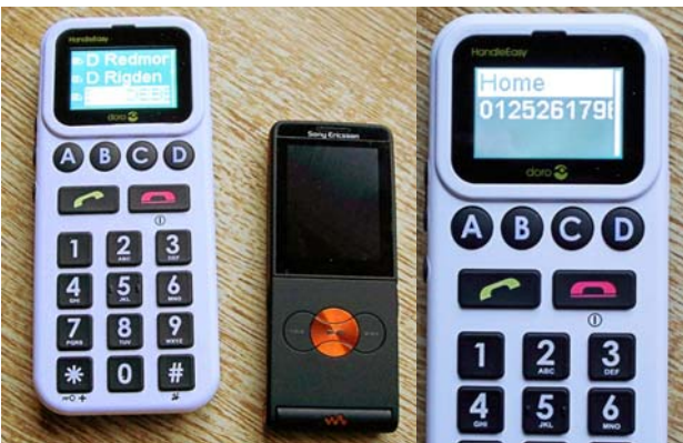
The Doro HandleEasy 328gsm compared with a current Sony Ericsson mobile and (right) four one-touch keys with Home number
