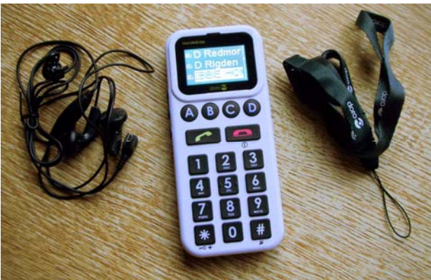
The Doro HandleEasy 328gsm with supplied earphone mic (left) and carry strap (right). Display shows phonebook entries.
