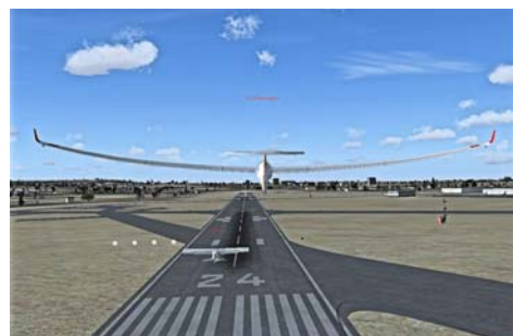
Airborne before and behind the tow plane and the wings curve upwards showing the aerodynamic load.
