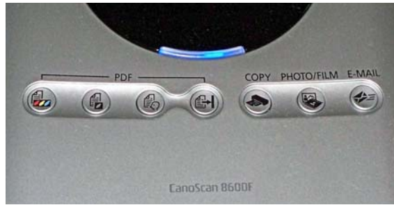
The EZ One-touch buttons. PDF scan choices left. Colour, black & white, e-mail. Main scan buttons right.
