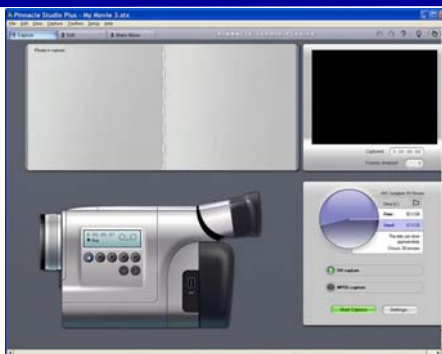
Fig. 1. The capture from Camcorder screen. When using a FireWire cable to connect the camera to the computer the on-screen mini controls control the camera — fast forward, fast back, play etc.
